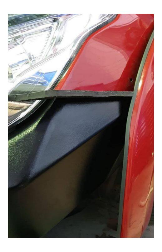
This will create an even gap on both sides, vs trying to align 1 side at a time. We also recommend using same foam under the head lights to maintain the correct gap.
